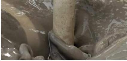
**Description of process generating the waste:** Oil and water-based drilling fluids are used to lubricate and remove drill cuttings during the drilling process. Drilling fluids are processed to remove solids and recirculated. When drilling is complete, or the drilling fluid is spent the drilling fluids are sent for disposal.
