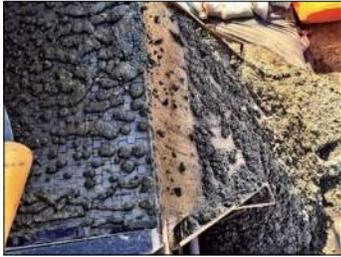
**Description of process generating the waste:** Small pieces of rock and soil (including spall and carvings) that break away from the well walls during drilling and are screened out of the liquid mud system.
