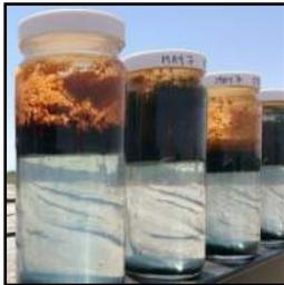
**Description of process generating the waste:** Water (brine) brought up from the hydrocarbon bearing strata during the extraction of oil and gas. It may include formation water, water that has been injected into the formation and any chemicals added down hole or during the oil/water separation process.
