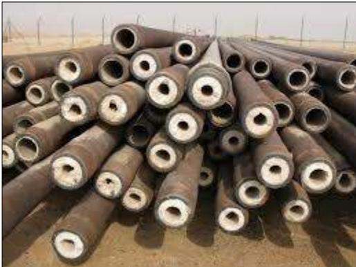
**Description of process generating the waste:** Scale or sludge containing Naturally Occurring Radioactive Material (NORM) or Technically Enhanced Naturally Occurring Radioactive Material (TENORM) typically removed from pipes, heater-treaters, tank bottom sludges, and other equipment. The scale typically consists of barium, calcium, or strontium sulfate that has precipitated out of solution in produced water along with radium, a radioactive nuclide.
