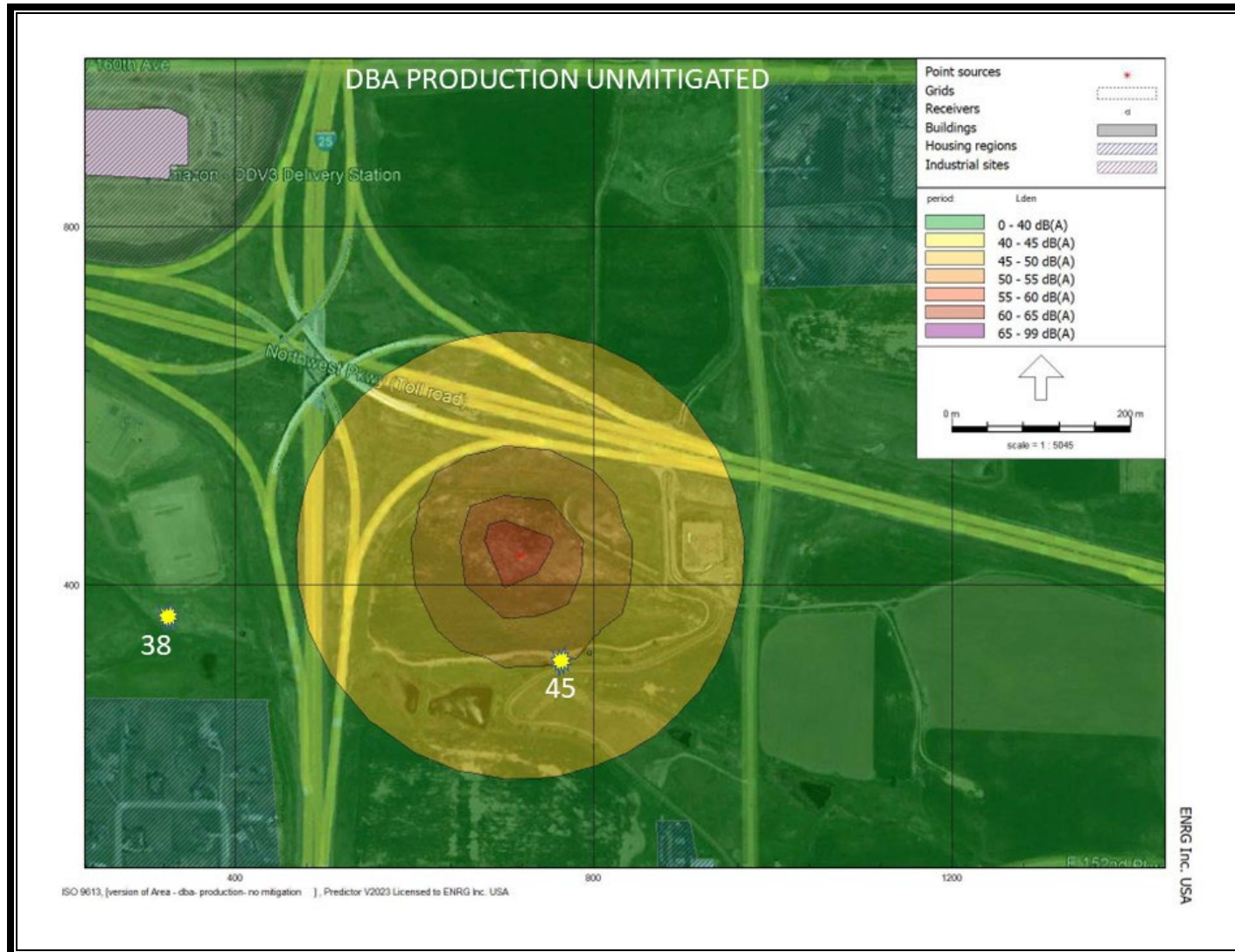
FIGURE 12. EXTRACTION OIL & GAS, INC. – WASHINGTON PAD SITE NOISE MITIGATION PLAN dB(A) PRODUCTION UN-MITIGATED SOUND LEVELS
