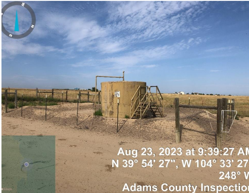
Photo#3 Produced water tank
