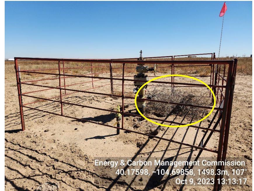
Photo 4: TA Wellhead, Debris
