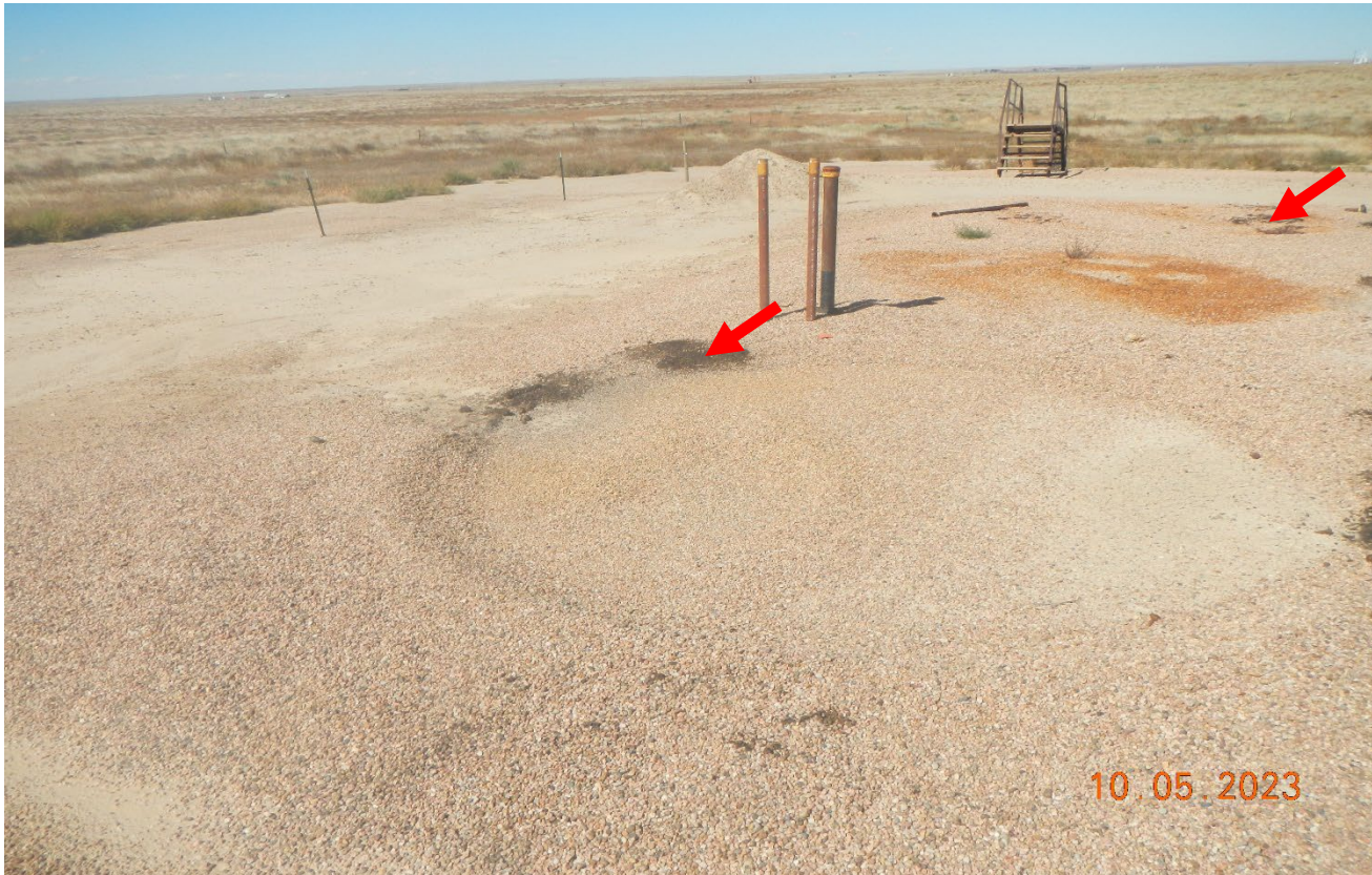
Photo 5. Facing northwest where tanks were located. There is oil impacted soils shown at red arrows.
