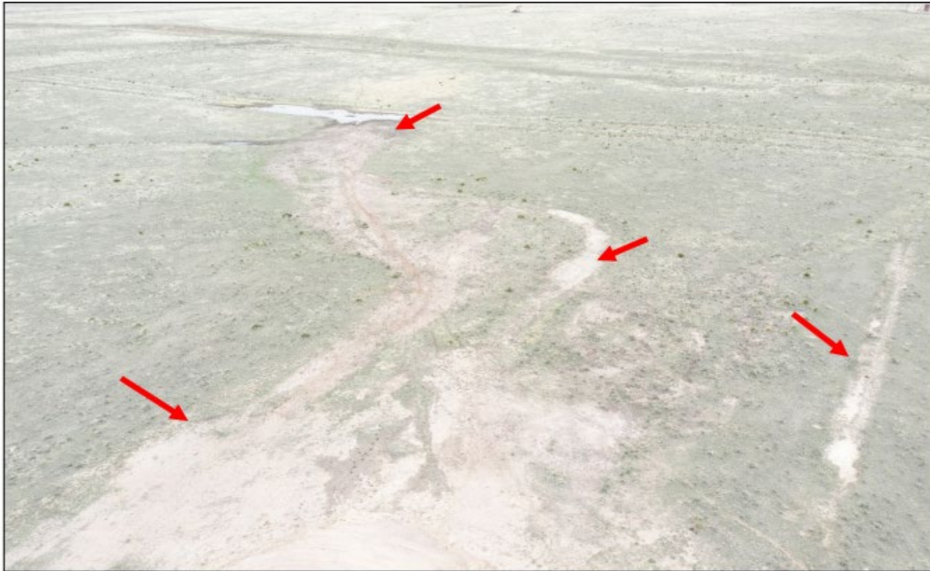
Photo 2. Drone aerial photo facing northwest from the Foster #1 wellsite. There is multiple impacted areas from previous spill. Site investigation and remediation will need to occur.
