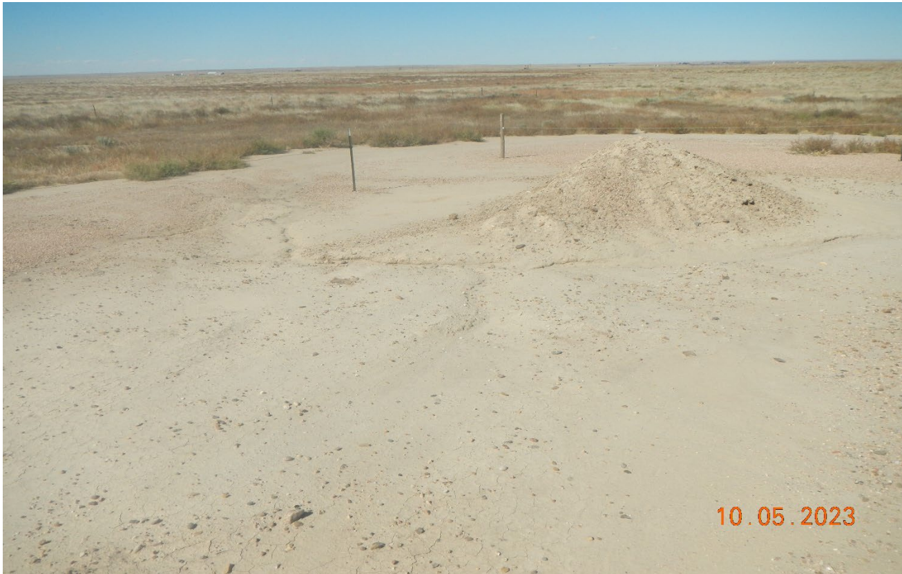
Photo 6. Facing toward the northwest side of the location. There is Stormwater erosion occurring off this area of the location. It appears impacted soils have been piled up and are not properly contained.
