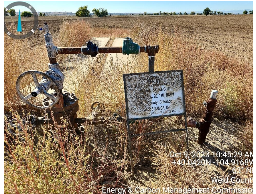
Photo 4 well head unused pumping unit pad
