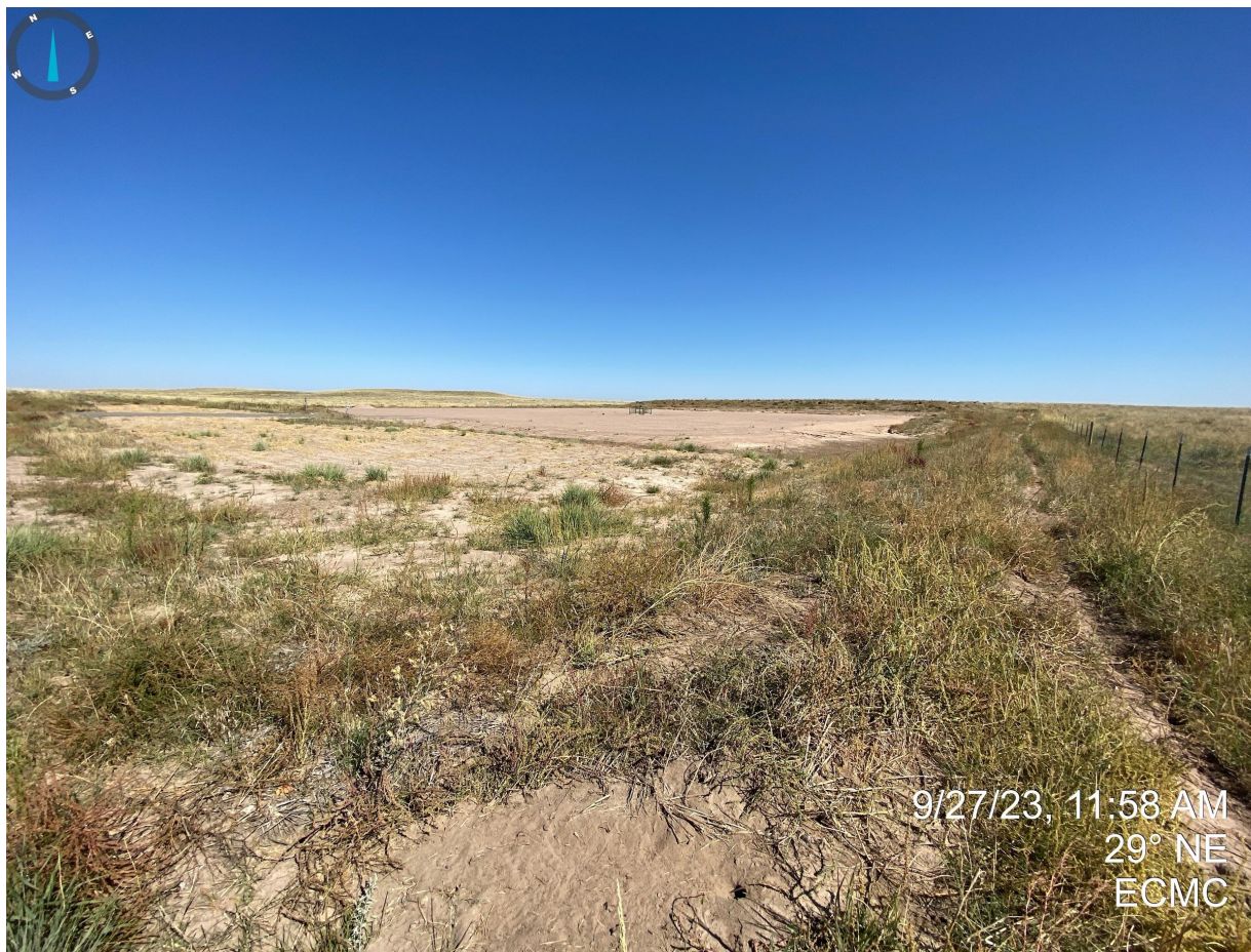
Photo 23. Taken from the southwestern corner of the location. Photo illustrates that the disturbance area is not properly stabilized against wind and water erosion (e.g. bare soils) and undesirable vegetation (e.g. kochia and russian thistle) appears to be unmanaged throughout.
