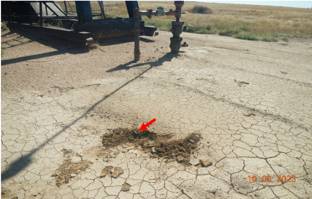
Photo 3. Facing toward the wellhead. There is oil stained soils. It appears dirt was placed over this area to cover up the impacted soils. Impacted soil need to be immediately excavated, cleaned up, and properly disposed per Rule 912.
