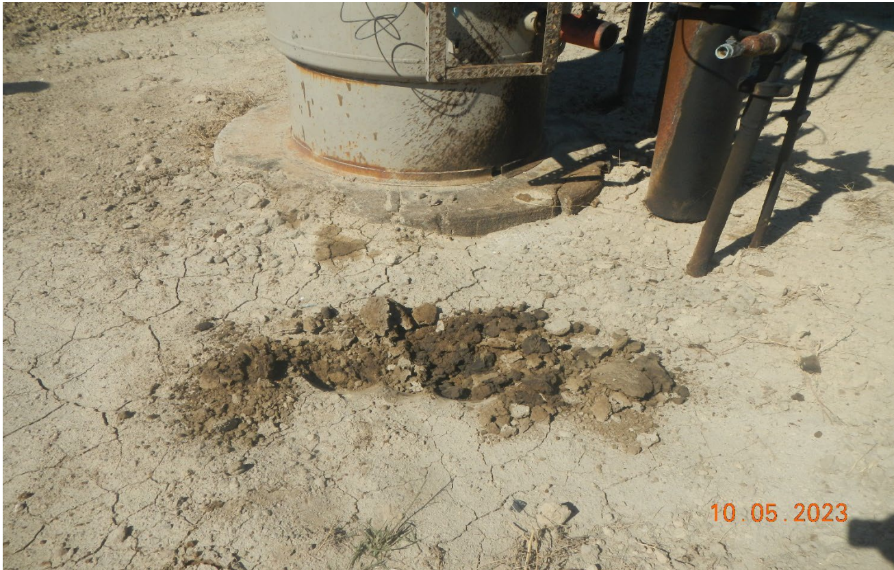
Photo 7. There is oil saturated soils that still remain at the separator. There was dirt spread over the stained soil to cover this spill. Impacted soil need to be immediately excavated, cleaned up, and properly disposed per Rule 912.
