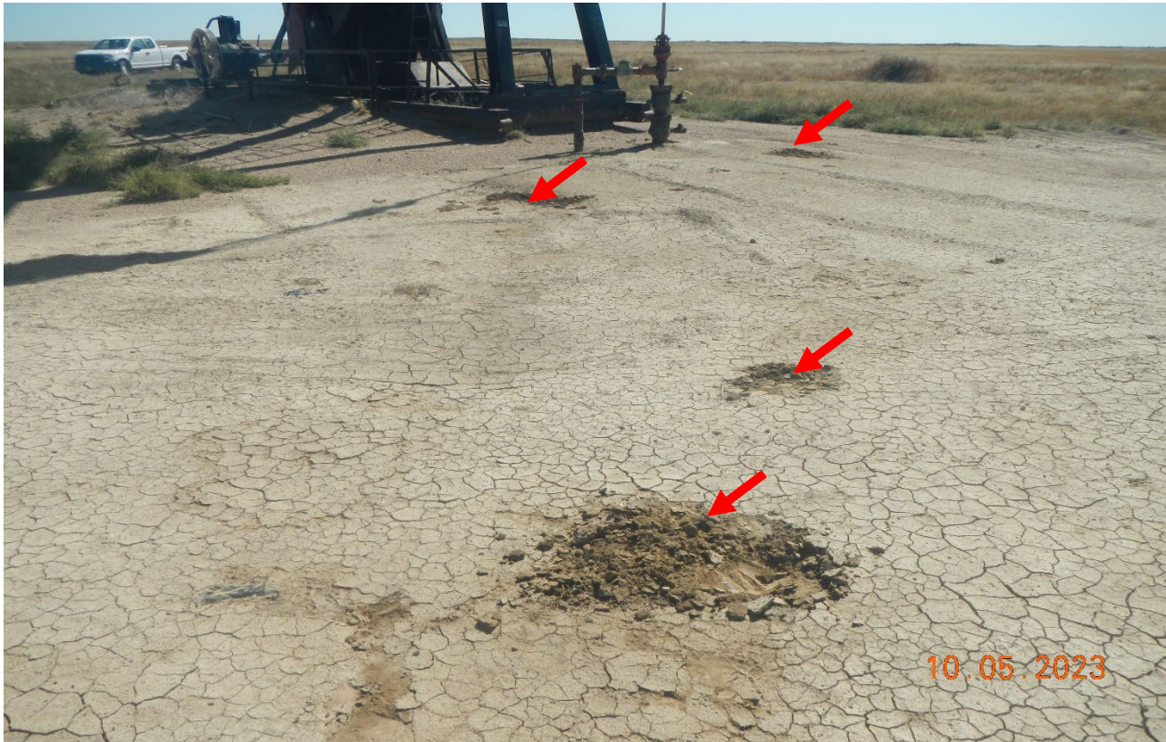
Photo 4. There is impacted soils that were observed in an area approximately 20x40 feet in size. After further investigation the spill appears to be reportable under 912.b. Red arrows point to areas of oil stained soils.
