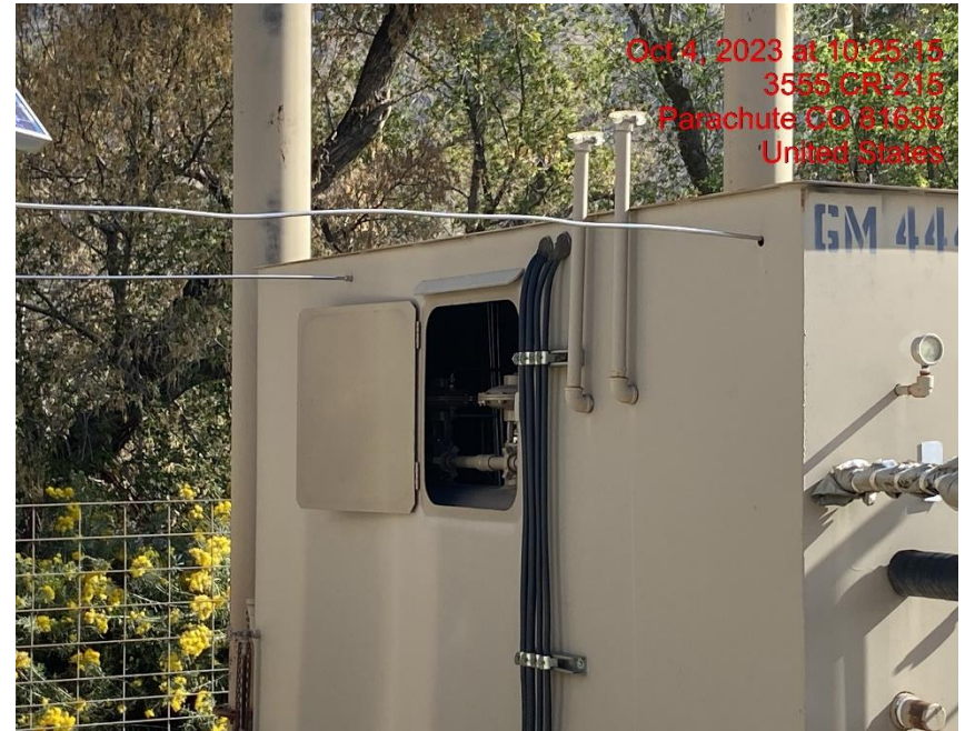
Unsecured Hatch on Separators – Photo #06769
