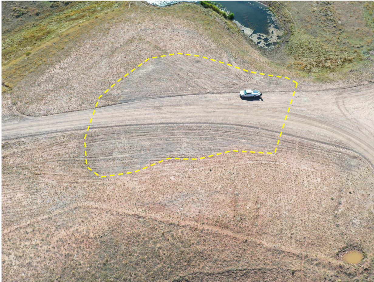
Photo 6: Photo taken with use of a sUAS. Yellow polygon represents areas where gravel/road base remain, and where reclamation is not progressing towards 1004 standards
