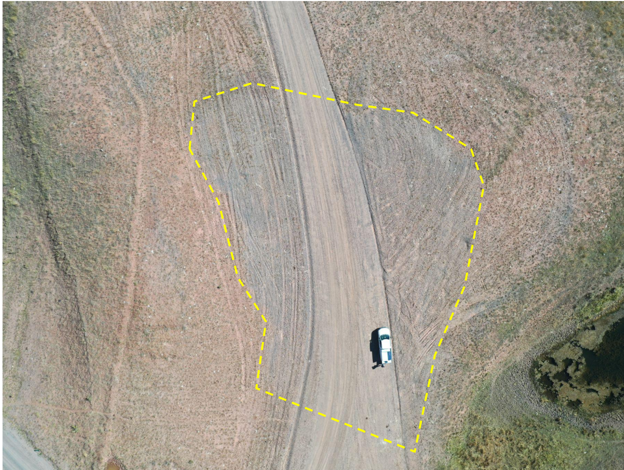
Photo 7: Photo taken with use of a sUAS. Yellow polygon represents areas where gravel/road base remain, and where reclamation is not progressing towards 1004 standards
