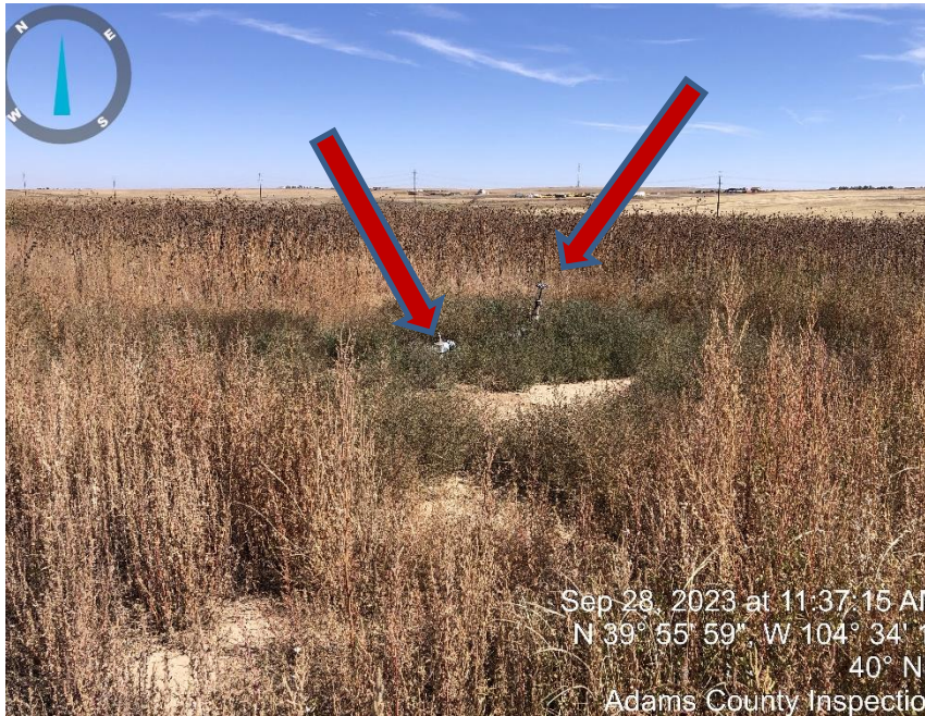
Photo #3 Unmarked risers / flow lines & weeds.
