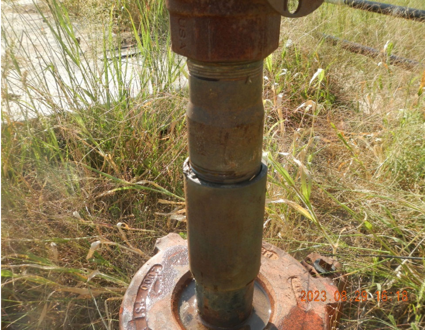
3. Gas leaking from collar and nipple connection.
