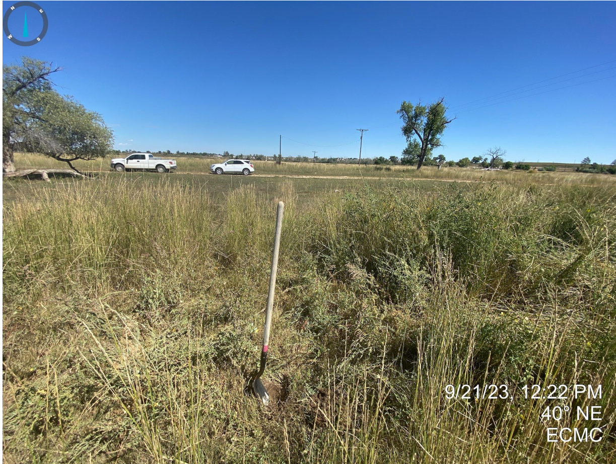
Photo 5. Taken south of the former location. Staff performed a compaction test in reference area soil and dug approximately 6" with minimal effort.
