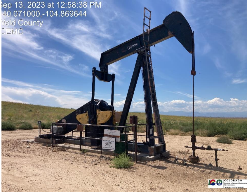
Pic 1 wellhead / pumpjack
