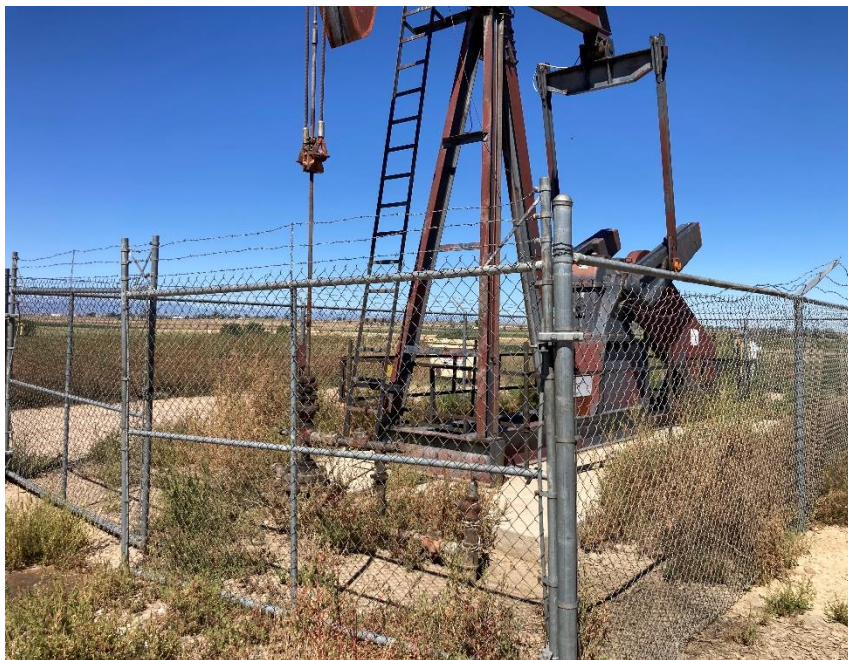
Pic 1 wellhead / pumpjack / weeds unmanaged.
