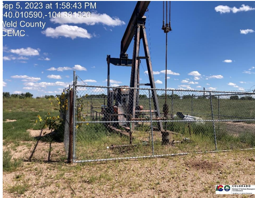
Pic 1 wellhead / pumpjack / weeds unmanaged on location
