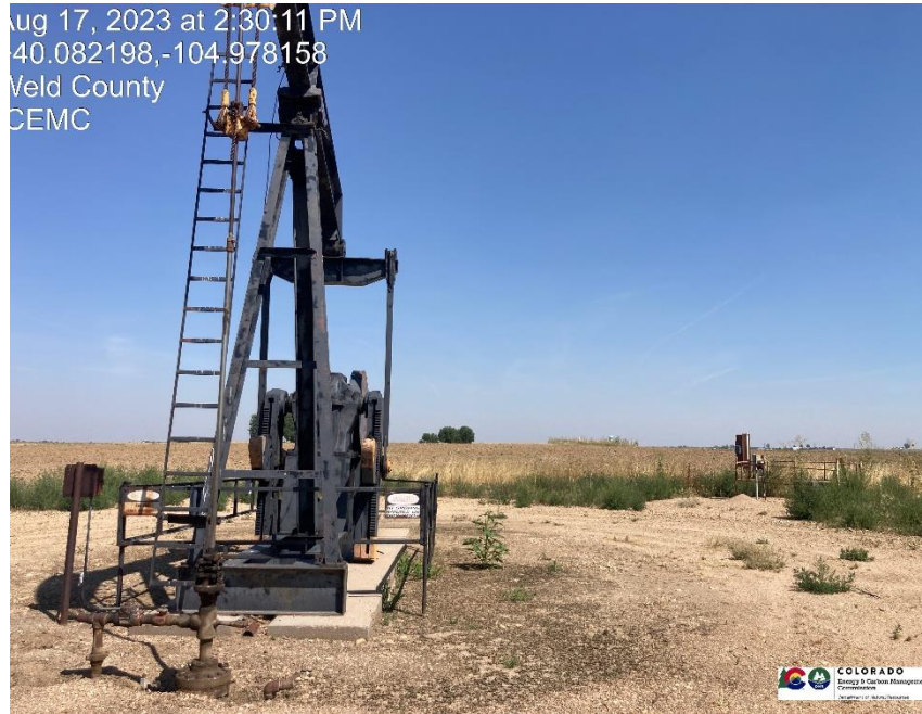
Pic 1 wellhead / pump jack
