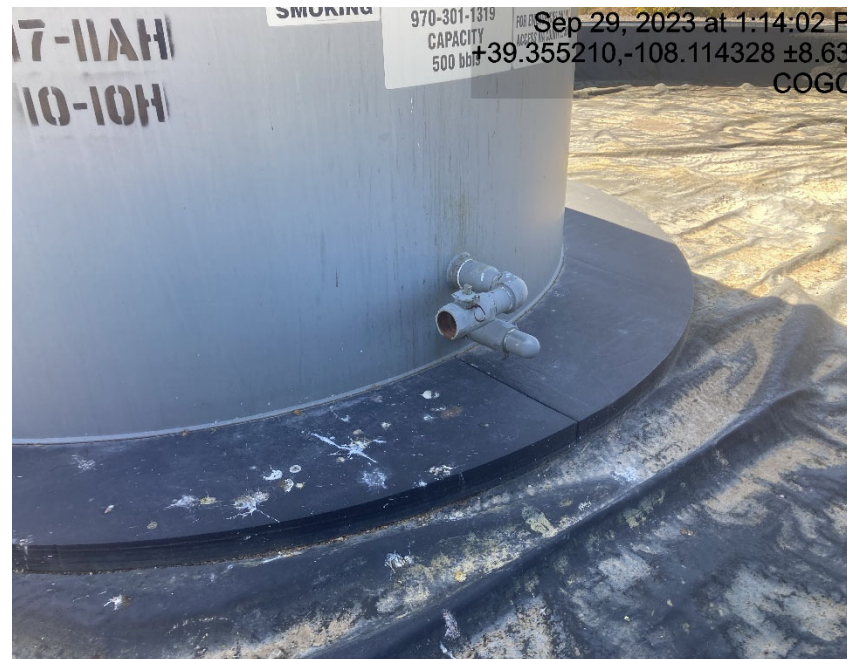
Tank missing cap/plug
