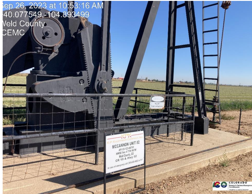
Pic 1 wellhead / pumpjack
