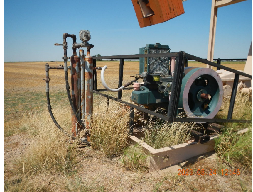
6. Prime mover and supply gas vessel. Note vegetation.
