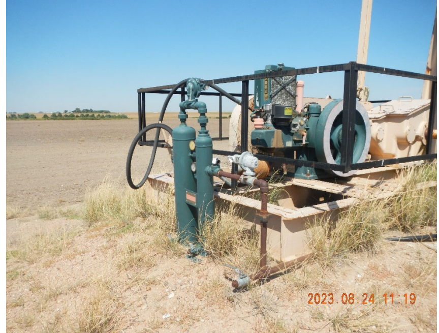
6. Prime mover and supply gas dryer vessel.
