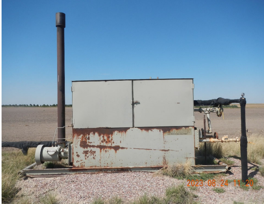
7. Horizontal heated separator.
