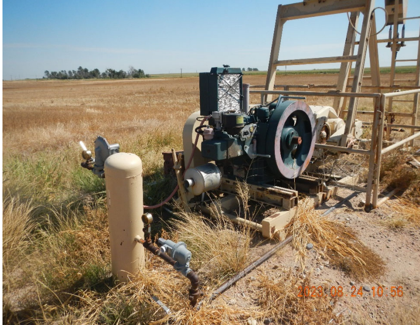
5. Prime mover and supply gas dryer vessel. Note vegetation.
