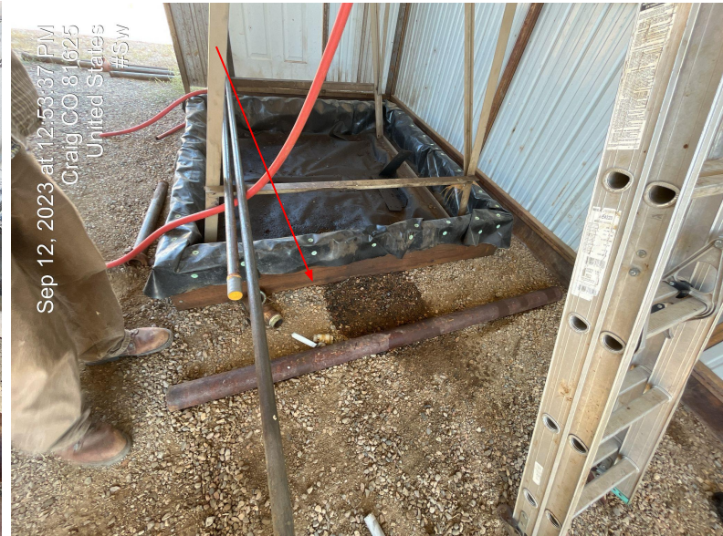
Photo 39 and 40. Stained soils found within shed underneath pipe (left) and underneath engine oil tank (right).
