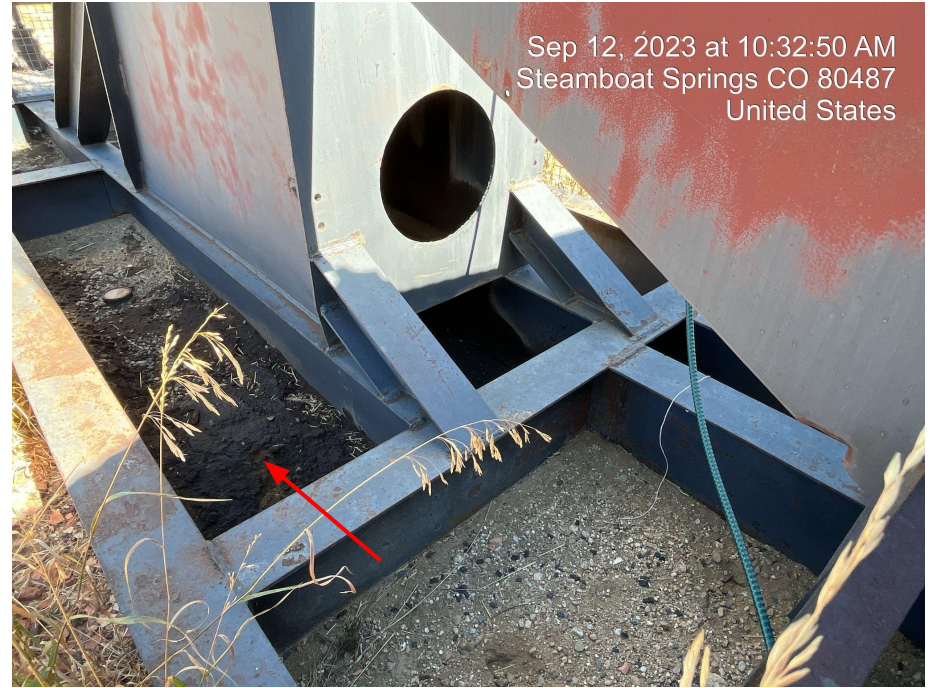
Photo 14. Stained soils observed around pumpjack.
