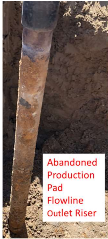
Figure 5- The Abandoned Well Flowline Inlet Riser
