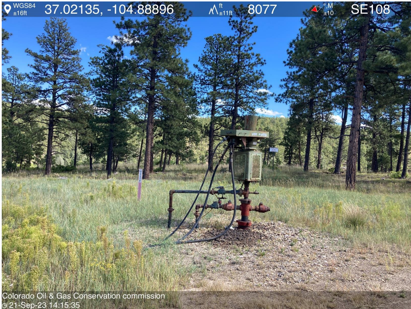
PHOTO 4: WELLHEAD/ AREA OF IMPACTED SOIL NEAR R WELLHEAD APPEARS TO BE FROM LEAKING HYDRO HOSES IN THE PAST, HOSED DID NOT APPEAR TO BE LEAKING AT TIME OF INSPECTION. Conduct maintenance on equipment, cleanup stained material and review self inspection processes. COMPLY WITH RULE 1002,(2).D (BE SURE TO INSPECT HYDRO HOSES AND CONNECTIONS FOR ANY LEAKS AND REPAIR. CA DATE 10-26-2023.
