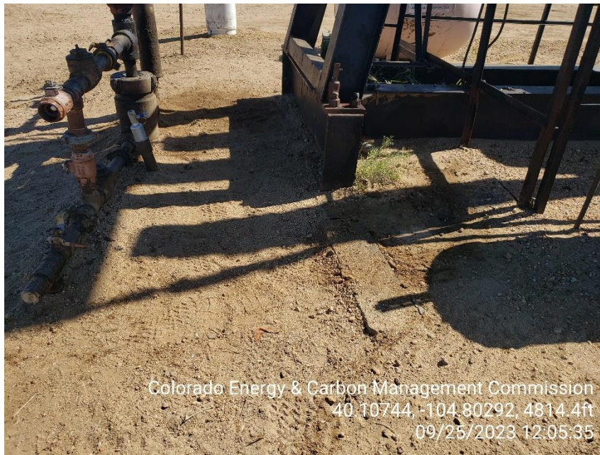
Photo 11 Stained soil around the WH and pump jack base.
