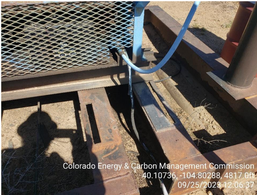
Photo 13 Stained soil under the pump jack engine skid plate.
