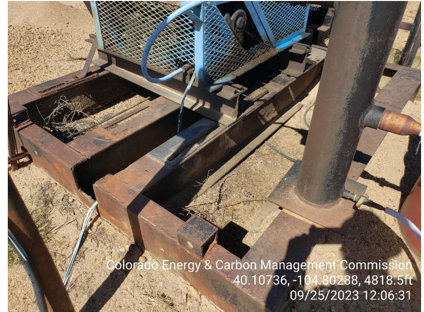
Photo 14 Stained soil under the pump jack engine skid plate.
