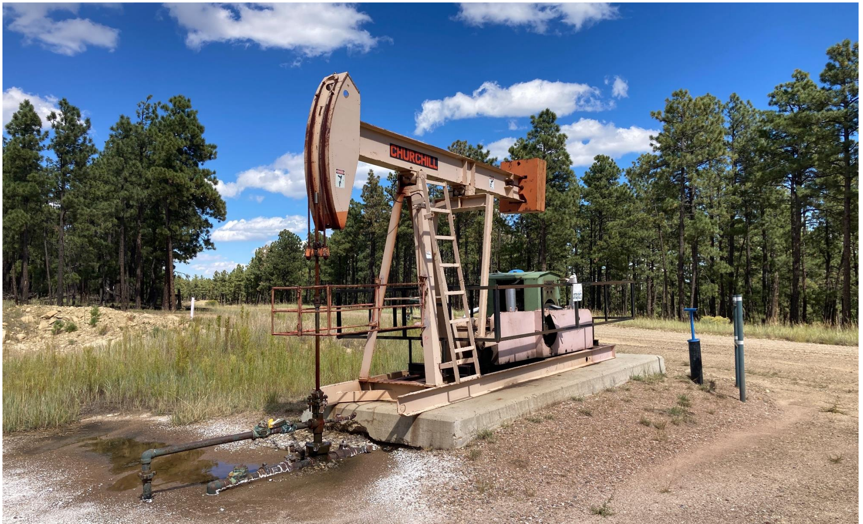
PHOTO 3: R WELLHEAD AND EQUIPMENT/ Produced water spill from the wellhead has left a salt impacted area around the wellhead. Securely fasten all valves, pipes, fittings, and Production Facilities to ensure good mechanical condition, inspect at regular intervals and maintain in good mechanical condition remove and dispose of impacted material per Rule 608.e. ca date 10-25-2023.
