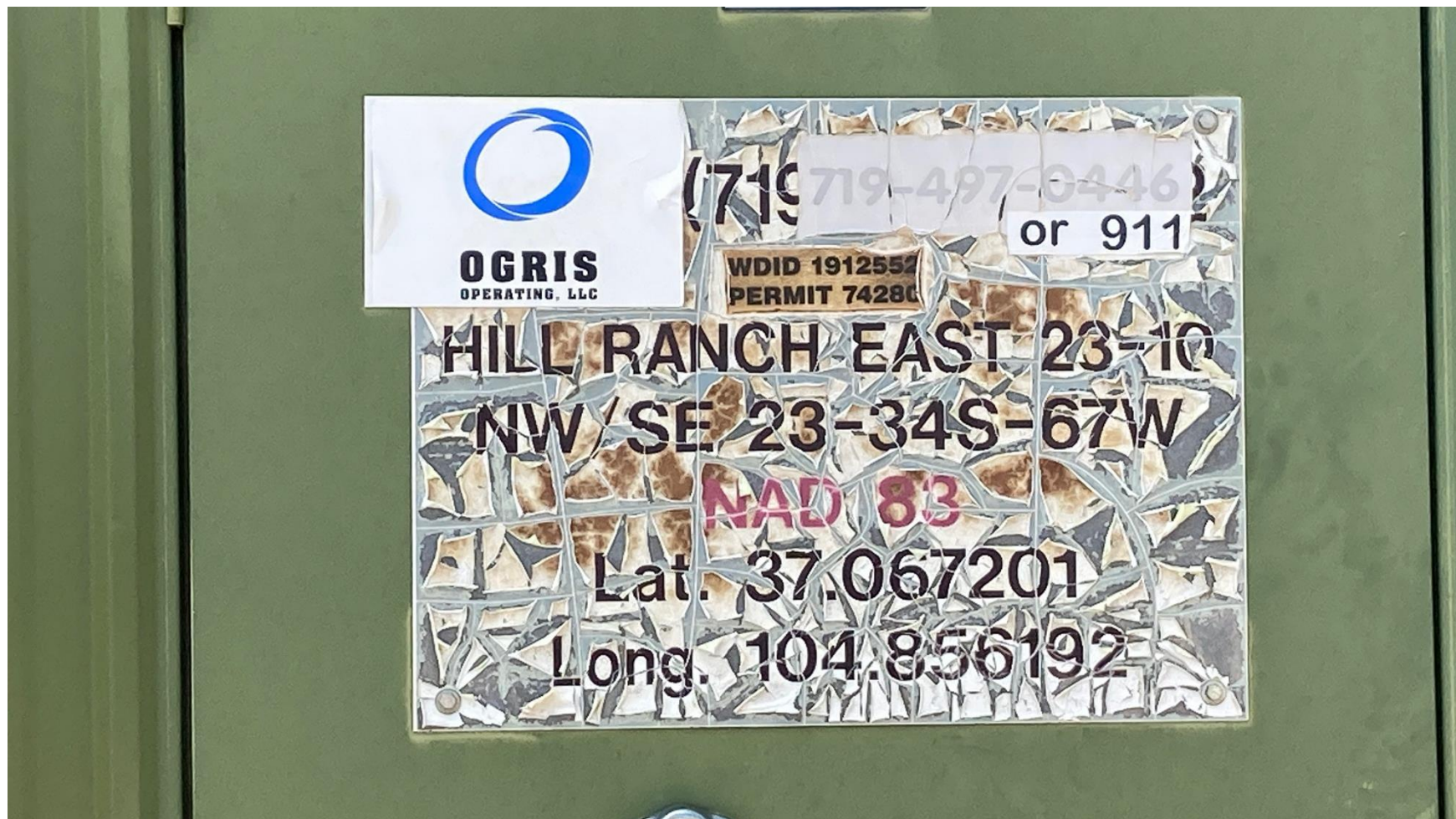
PHOTO 1: WELL SIGN CRACKED AND FADED. POST SIGN PER RULE 605, BE SURE TO INCLUDE ALL NEW SIGN REQUIREMENT LIST IN THE NEW RULES (605). CA DATE 10-25-2023.
