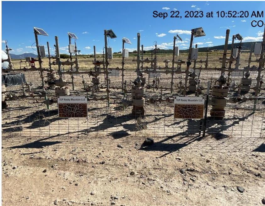
Photo # 230 RWF 313-23 & 413-23 wellhead signs weathered & illegible.
