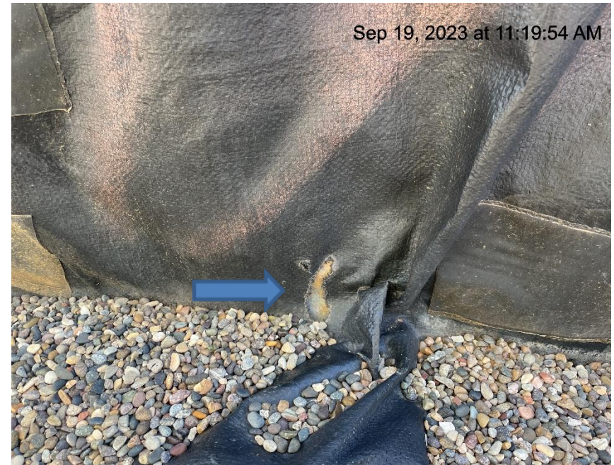
Photo # 9856 Hole in secondary containment liner
