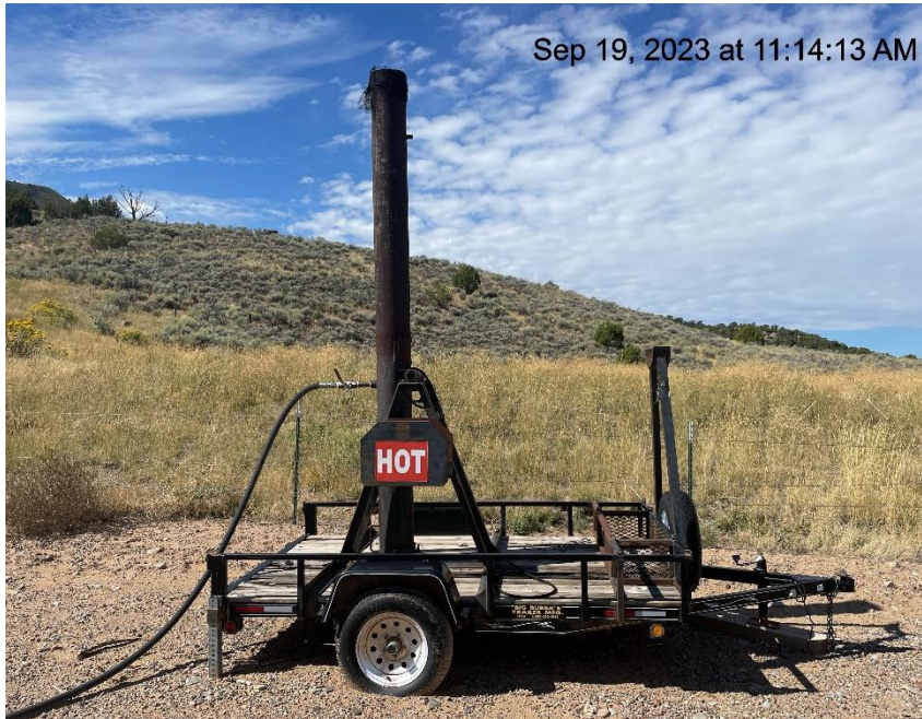
Photo # 9861 Flare lacks auto-igniter or continuous pilot light
