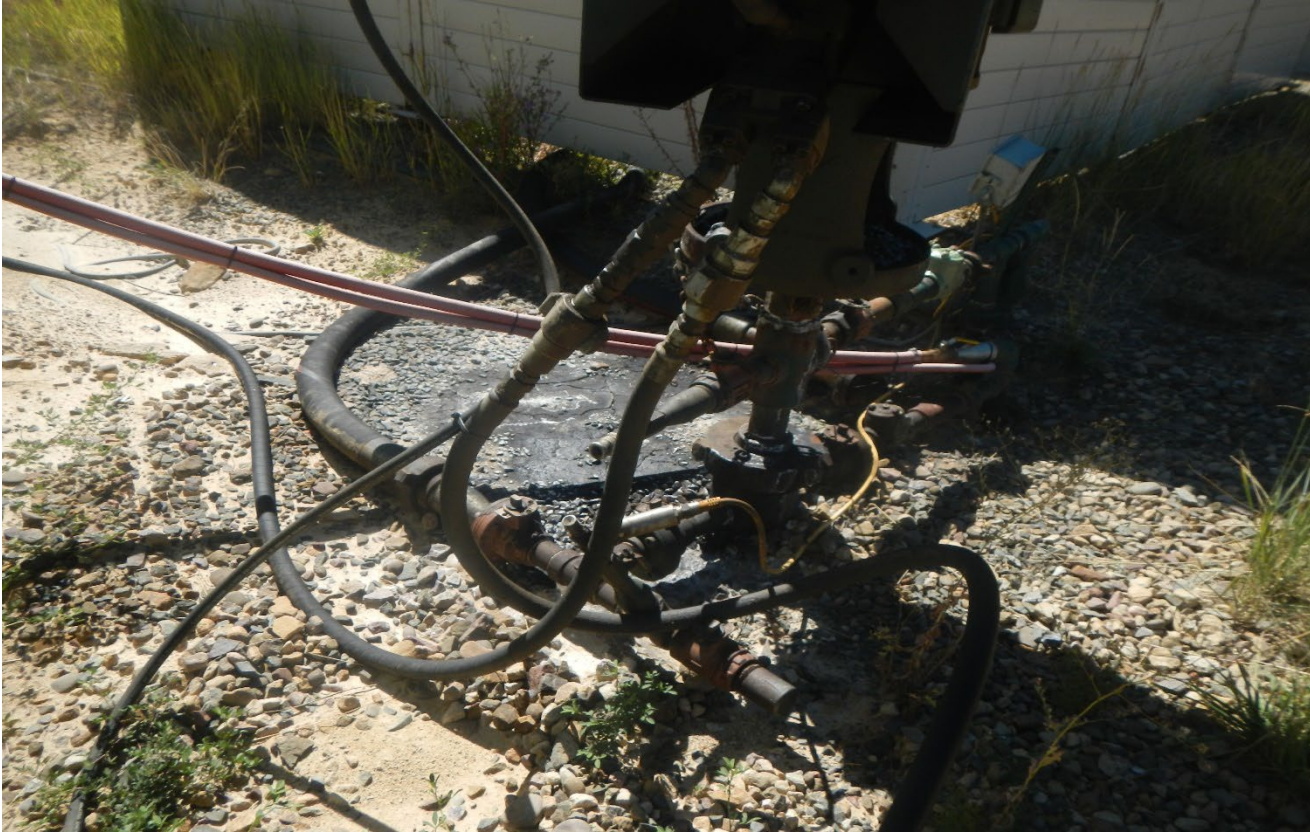
Photo 4. There are stained soils at the wellhead that need to be cleaned up.
