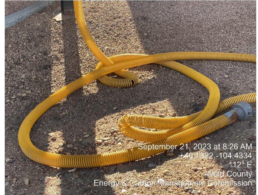
Weathered/ Ripped Vapor Line hose
