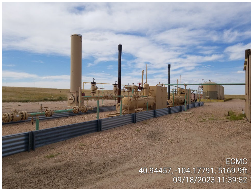
Photo 7 – Separators and ECD
