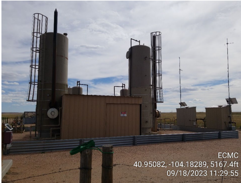
Photo 5 – Heater Treaters and Gas Meters
