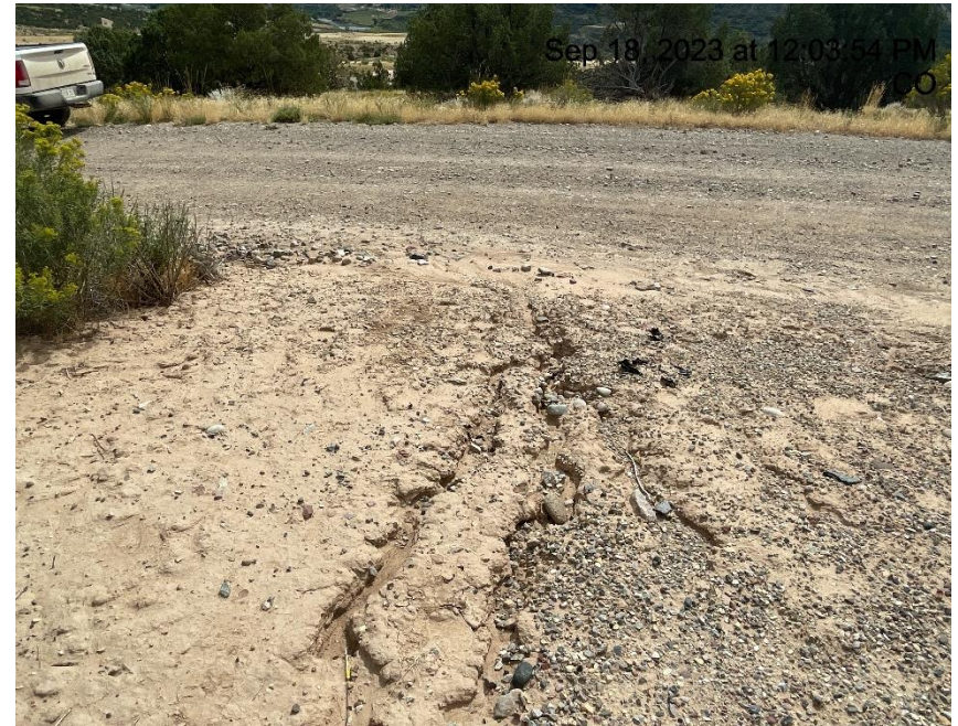
Photo # 9728 Erosion & transport of sediment off location/insufficient BMP's
