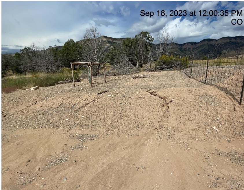
Photo # 9713 Erosion & transport of sediment off location/insufficient BMP's
