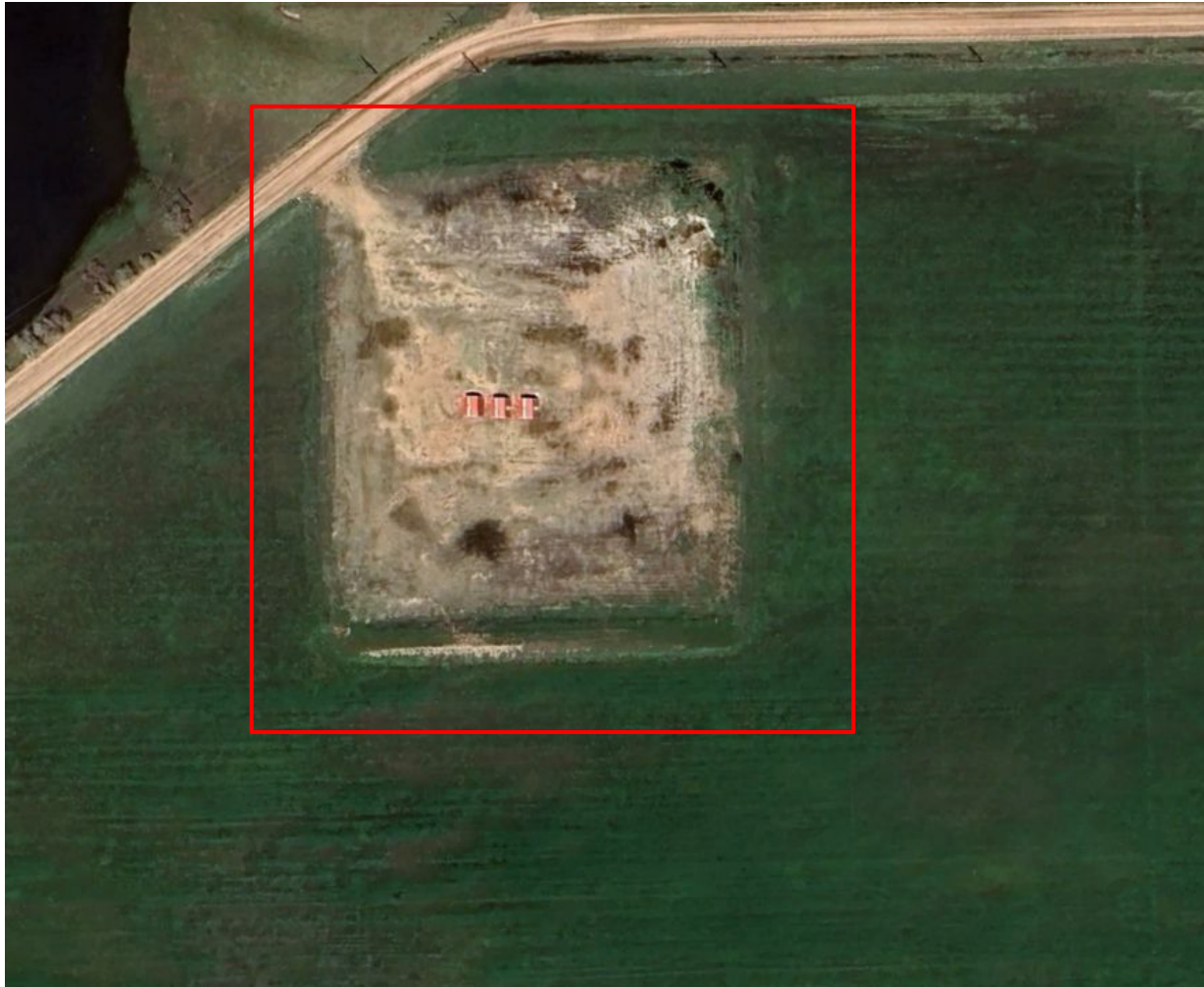
Photo 1. Google Earth aerial imagery from 5/16/2023 illustrating the location. Operator has failed to perform interim reclamation around the well location (red polygon).
