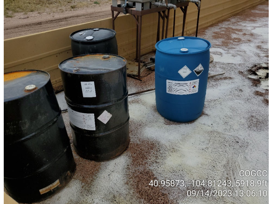
Photo 4 Salt crystals along south side of secondary containment
