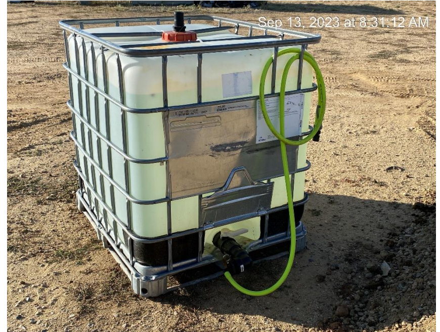
No spill containment
