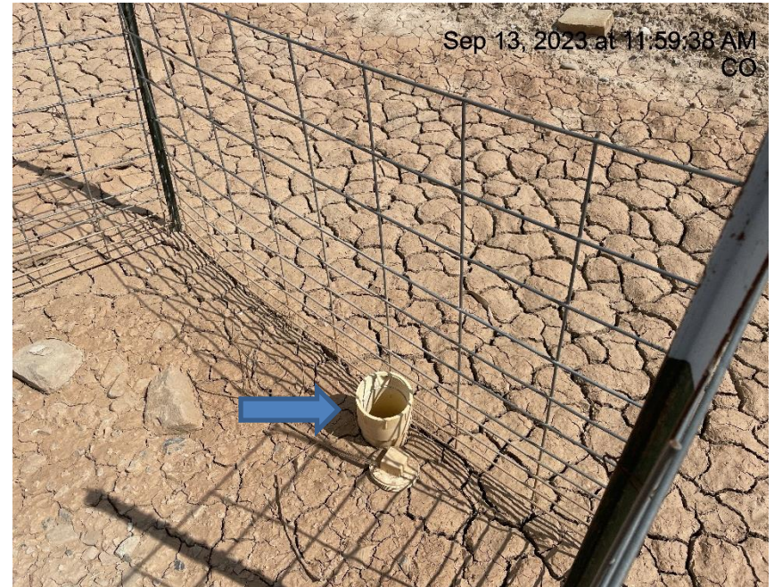
Photo # 9095 Open ended pipe/wildlife hazard
