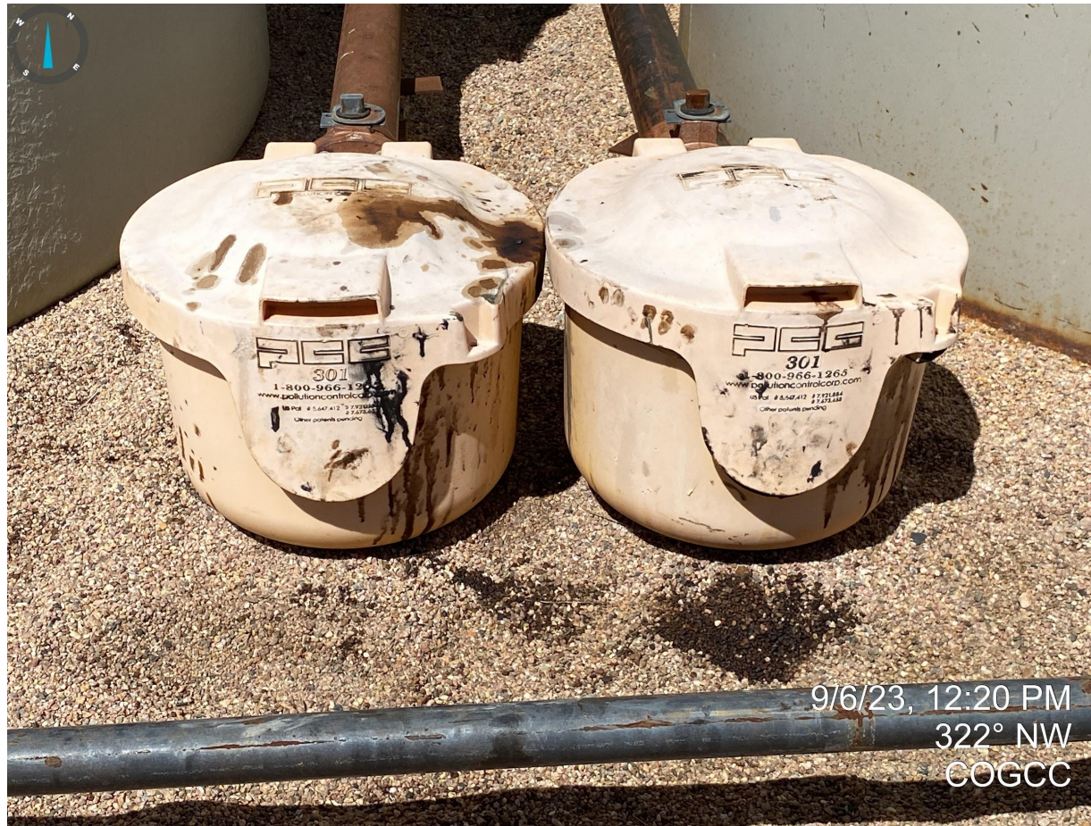
Photo 17. Stained soil at loadout lines.
