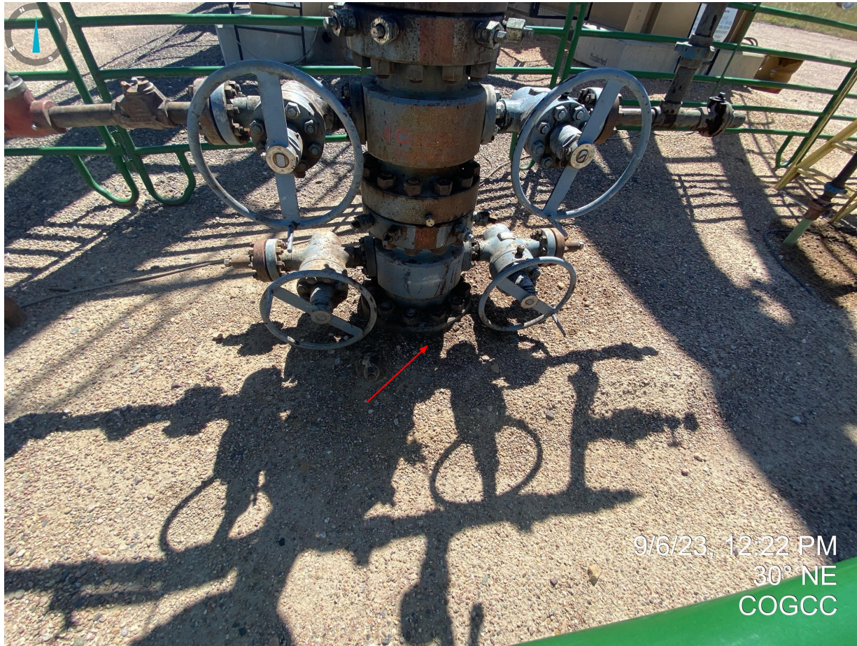
Photo 19. Stained soil at wellhead.
