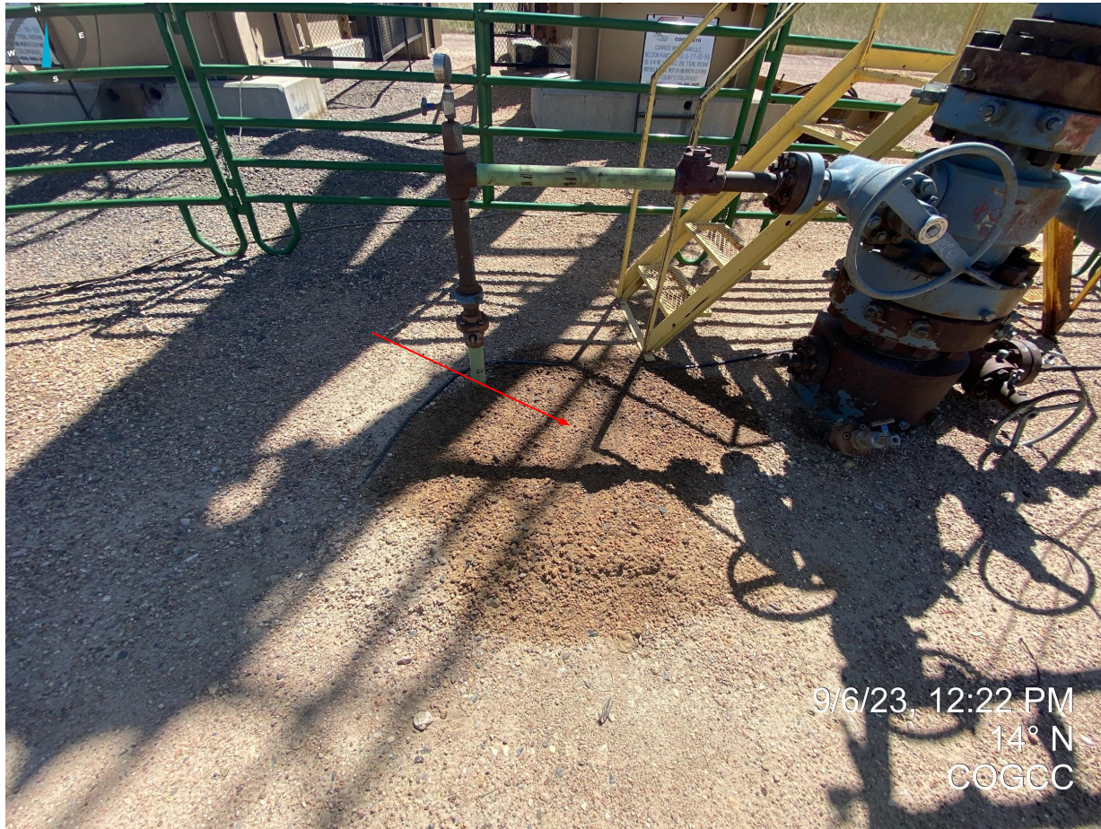
Photo 18. Stained soil at wellhead.
