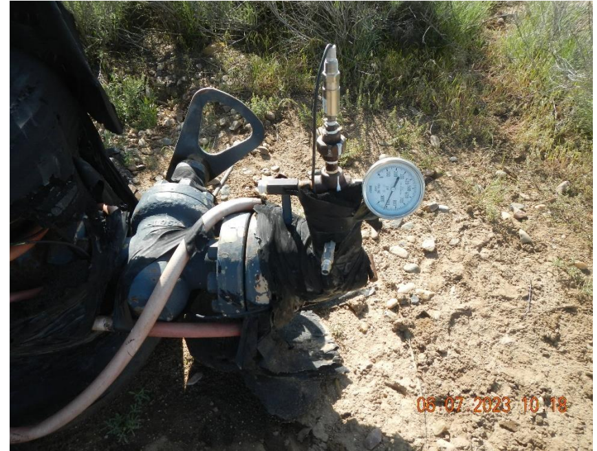
Production casing pressure was read as 901 psi.
