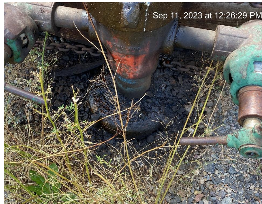
Staining. No Bradenhead access
