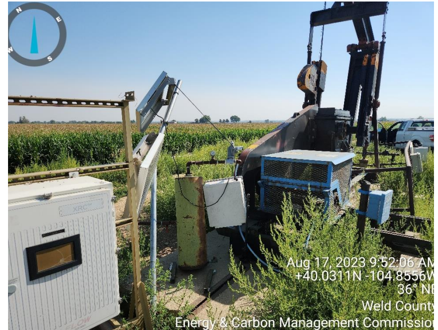
Photo 4 mechcal equipment in disrepair, no motor
