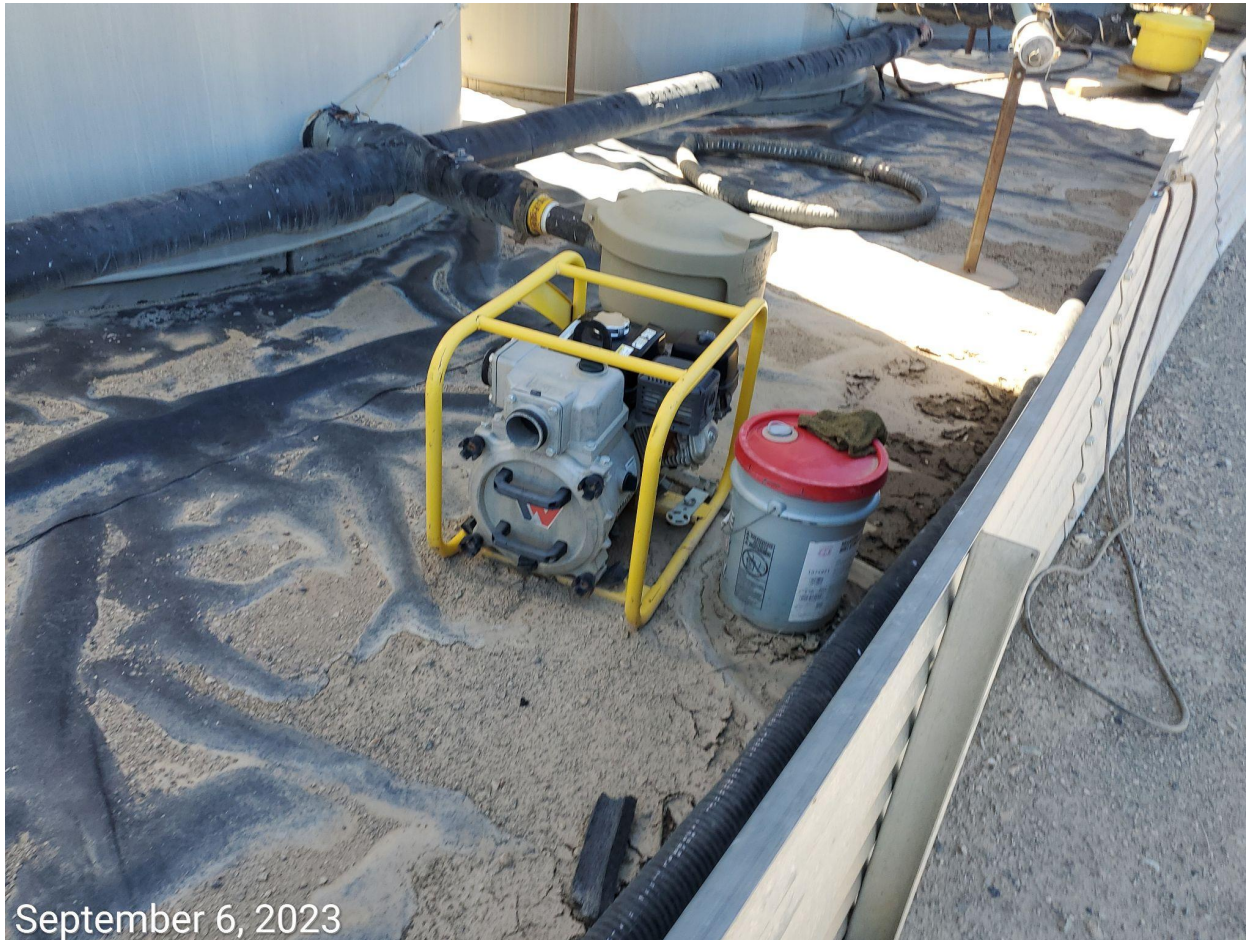
Photo 4: Unused equipment improperly stored within the secondary containment BMP.
