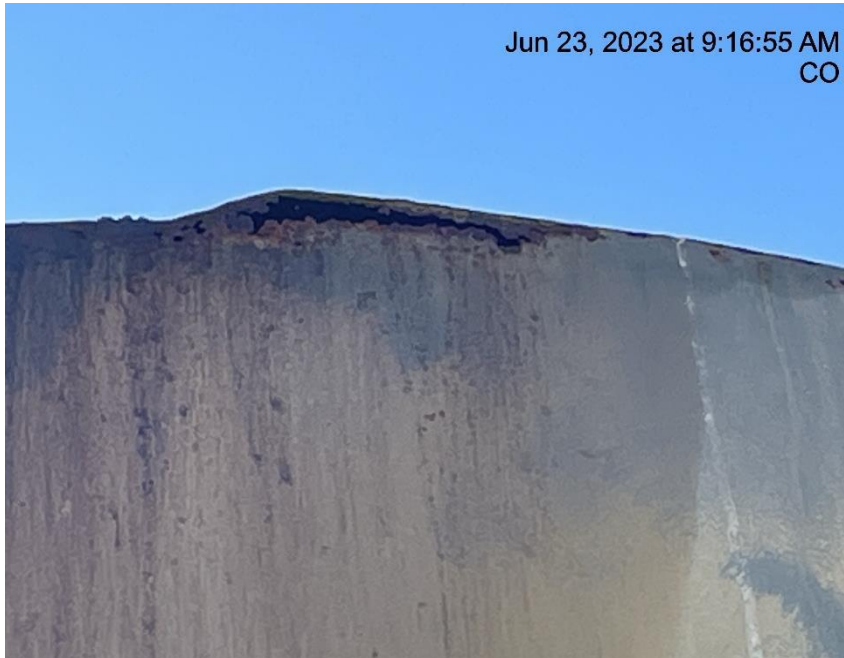
Photo # 1503 From inspection 708900837 conducted on 06/23/2023 Hole in production tank/tank corrosion
