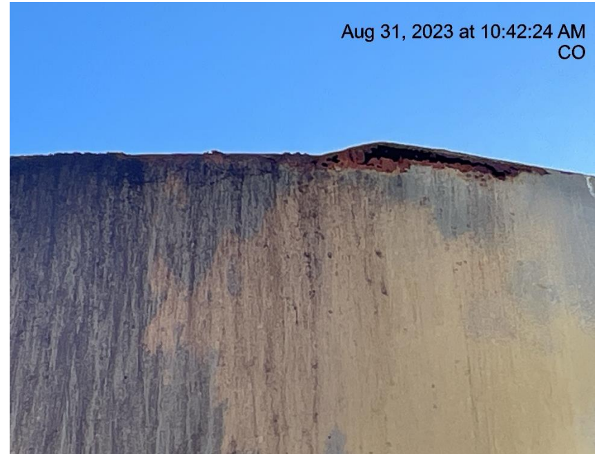
Photo # 7825 Hole in production tank/tank corrosion
