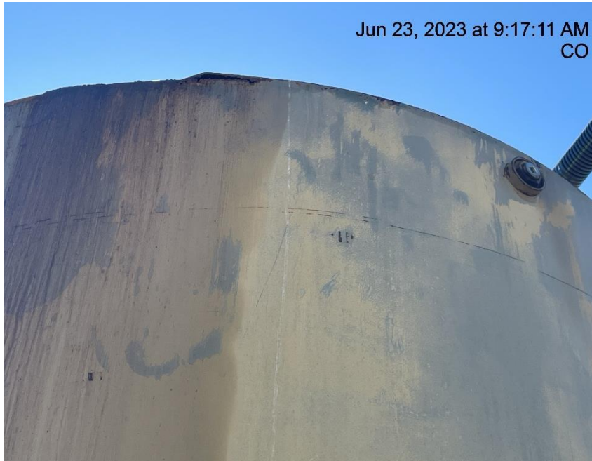
Photo # 1505 From inspection 708900837 conducted on 06/23/2023 Hole in production tank/tank corrosion
