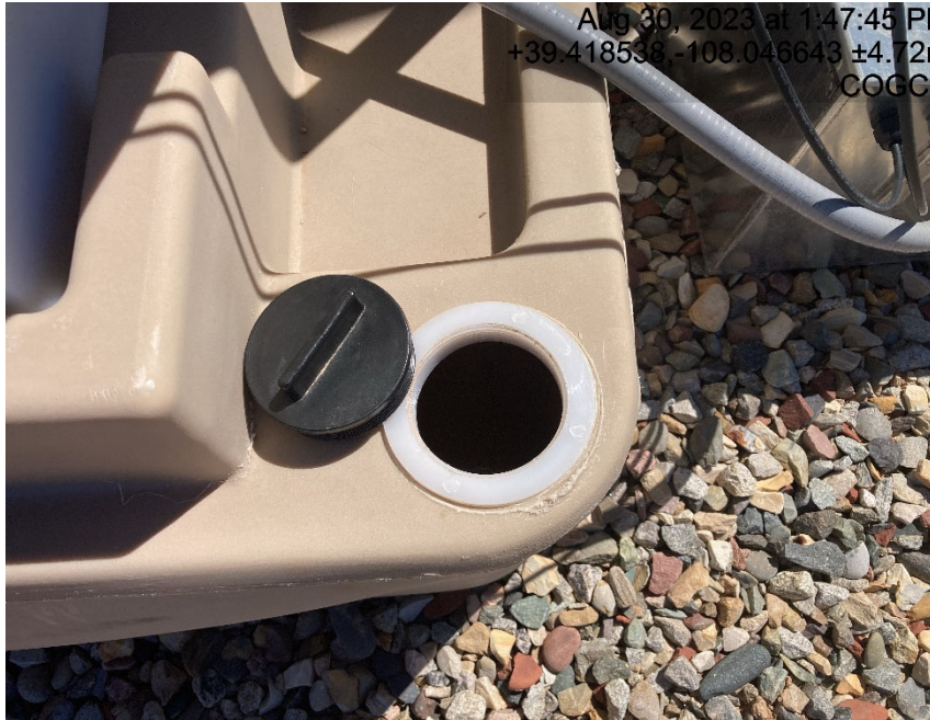
Chemical tank containment is full of fluid
