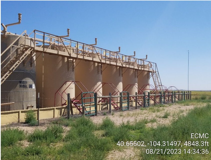
Photo 5 – Tank Battery
