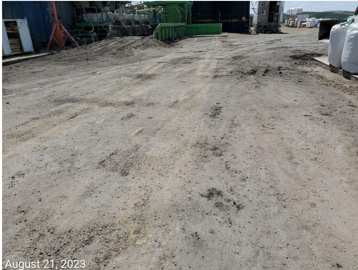
Photo 8: Drill cuttings area. Impacts remain apparent to the WPS. BMPs to mitigate impacts not apparent.
