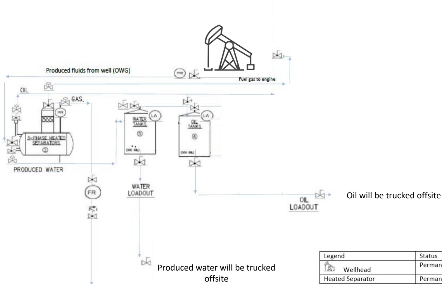
All gas piped to processing plant and separated there.
